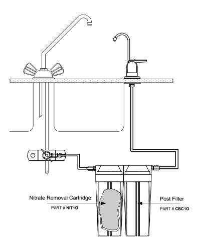
This system comes with all parts essential to installation. Easy to install, the 3 component system ensures pure healthy water for households with Nitrate problems. The water flows past a specially designed Nitrate removal cartridge ,then through a 0.5 micron carbon block cartridge to remove bad tastes, odours, other harmful chemicals ,plus giardia and cryptosporidium. Finally, water flows up through a dedicated tap on the benchtop.
